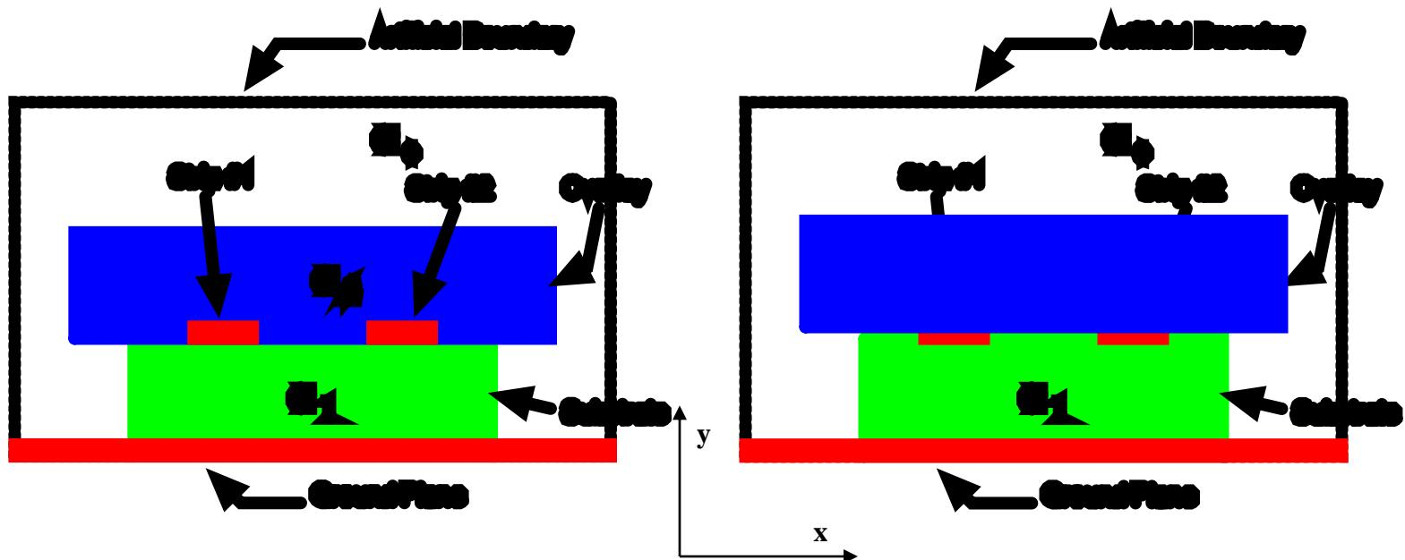
Coupled Microstrip lines with dielectric overlays with and without air gap due to the thickness of the conductors.
