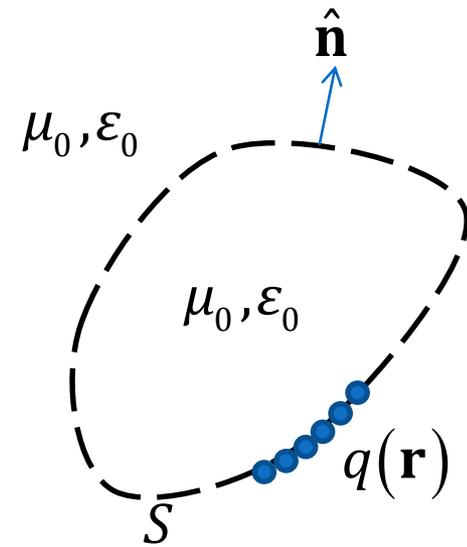
It is required to find the electric potential everywhere in space due to a PEC (cylinder) charged to a constant potential  $V_0$ .
