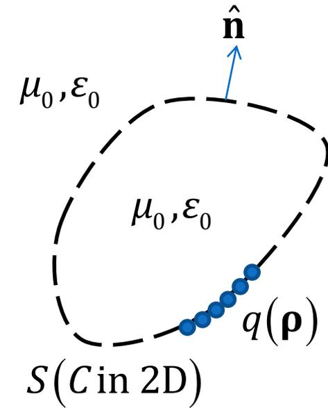
The above operator (integral) equation should be solved to determine the unknown charge distribution.
